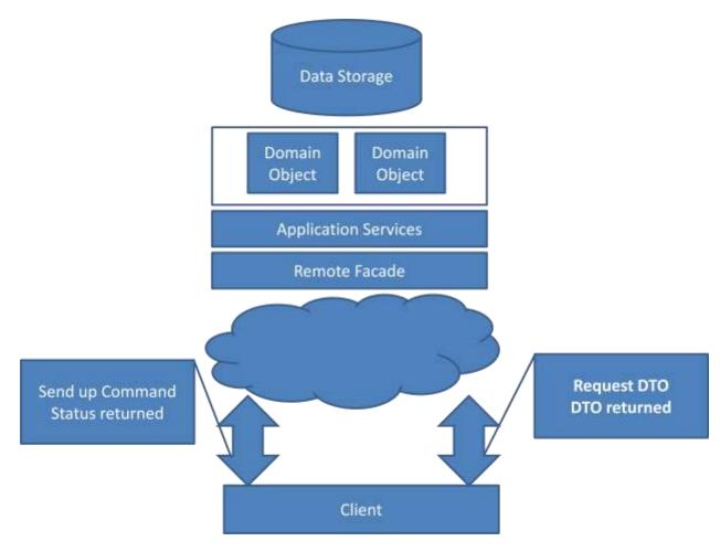
Figure 26 Stereotypical Architecture Sending Commands
