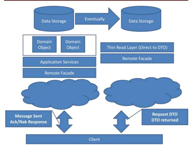
Figure 12 Separated Data Models with CQRS
